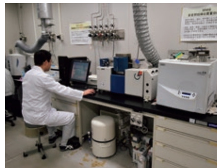
安定同位体比測定装置を用いた食品の原産地判別 Determining geographical origin of foods by using IRMS
